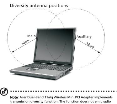
**Note:** Acer Dual-Band 11a/g Wireless Mini PCI Adapter implements transmission diversity function. The function does not emit radio frequencies simultaneously from both antennas. One of the antennas is selected automatically or manually (by users) to have good quality of radiocommunication.
